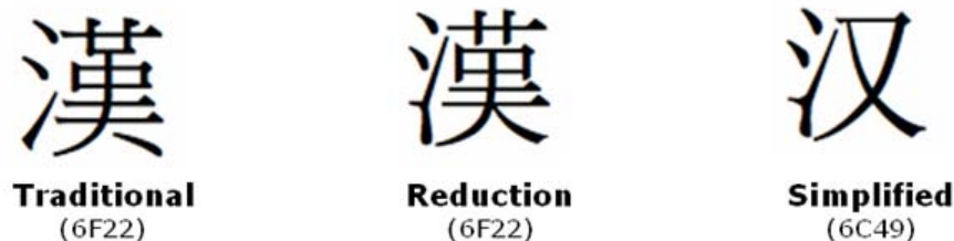
Figure 8. The Chinese character for "Han" literally means "Chinese," and is rendered via different glyphs among the three character sets. With Han Unification, the Traditional and Reduction style characters share the same Unicode encoding value.
